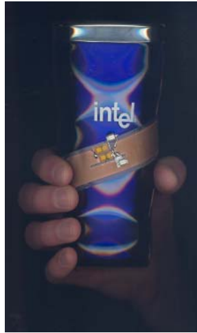
Fig. 2. The \alpha -Wisp mounted on a coffee cup. One application of Wisp sensors is tracking human activity by object use. (Figure reprinted from [1].)
